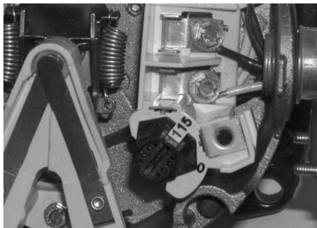
Figure 4: Motor Set for 115 Volt Operation
